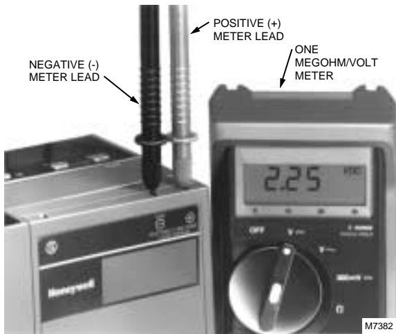
Fig. 11. Measuring flame signal voltage of 7800 SERIES controls.
