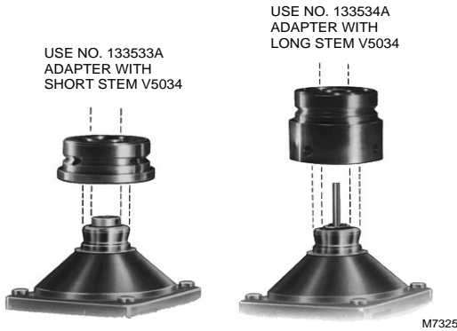
Fig. 3. Use adapters to connect V4055 Actuator with V5034 Valve.
