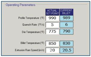
1. On each billet, **key process parameters** are monitored and adjusted to the specified recipe values enabling more consistent operation of the press by each operator on each shift.
